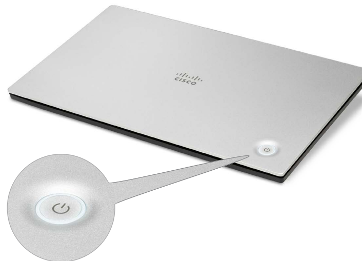
Power button with LED indicator
